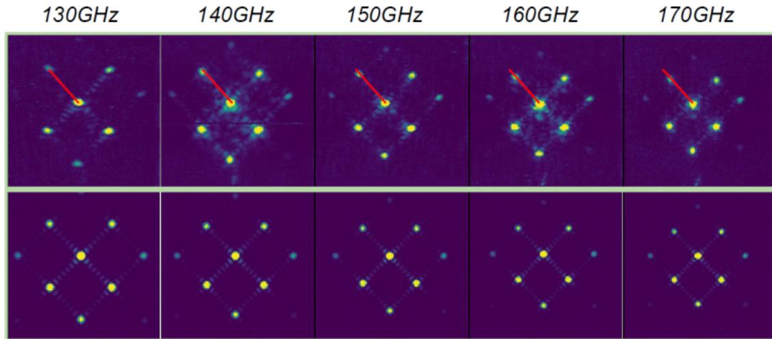
**Fig. 6.** Upper row: real measurements with TD. Lower row: Theoretical SB. Redline is a rule to see easily how the secondary peaks close to the center when the frequency rises as is expected.
