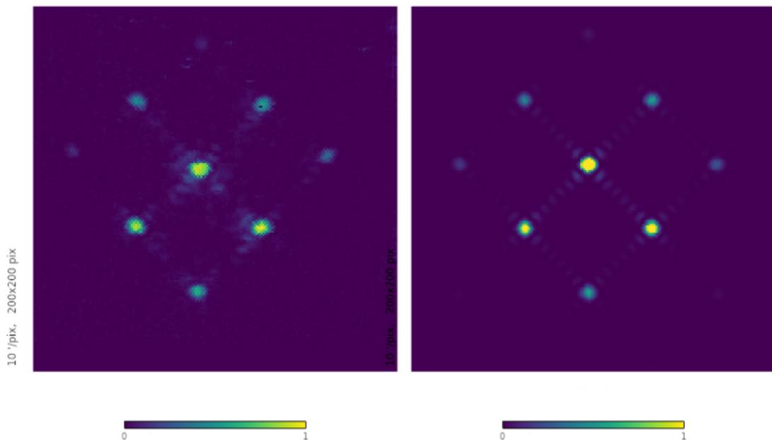
Comparison between the synthesised beam measured with one of the TES in the technological demonstrator (left panel) and the predicted beam without aberration effects (right panel).
