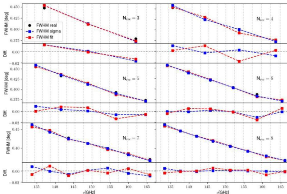
**Fig. 7.** Angular resolution (FWHM) measured with two independent methods (*sigma* in blue and *fit* in red lines). Dashed line shows the frequency used to simulated the TOD in simulations. Black dots are represents the theoretical angular resolution in the frequencies of sub-band reconstruction.
