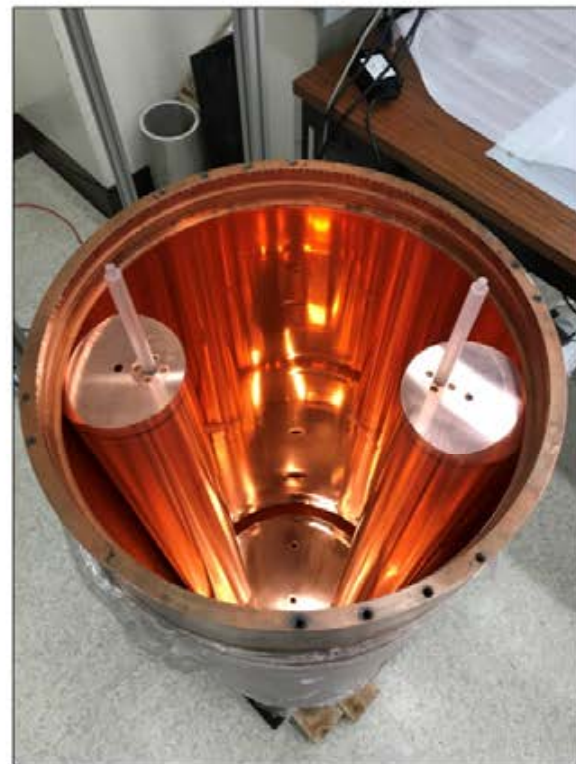
Cavity from run 1c & 1d Larger 4.5" (then 6") diameter tuning rods 780 – 1200 MHz
