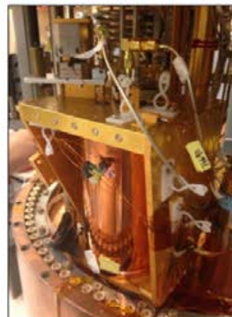
Sidecar Cavity 4-6 GHz TM_{010} mode > 7 GHz TM_{020} mode
