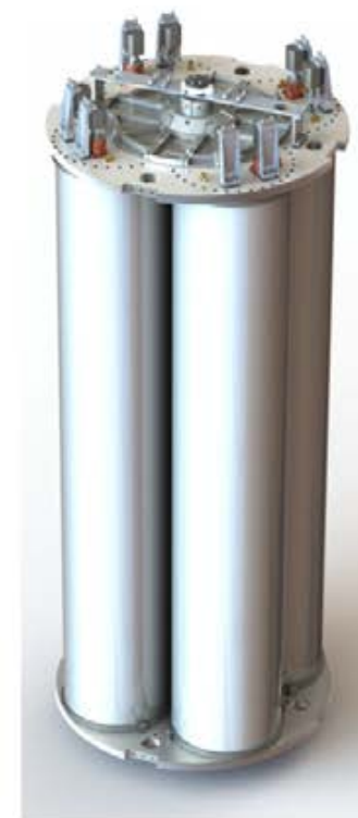
Cavity system for run 2a Full sized 4 cavity array Sapphire (1200 – 1500 MHz) Metal Rods (1500 – 2000 MHz)
